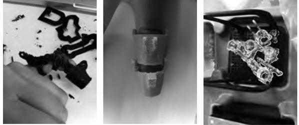
Figure 12. Printed Process whit PLA material, 13. Innoflex Flexible material, 14. Clear resin 3D printed material.
