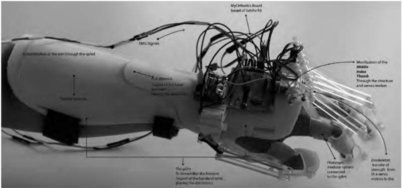
Figure 1: Development from the sketch to the final prototype using traditional and digital prototyping technique to produce MyOrthotics.
