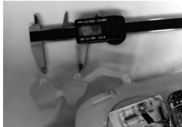
Figure 15. 3D Printed Thumb phalanges testing the accuracy and calculating the size of the exoskeleton connections.
