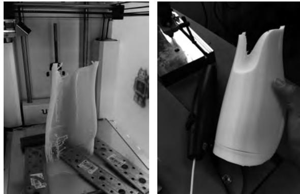
Figure 17. 3D Printing Process of the flexible part of the splint.
