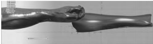
Figure 4. Free Form in 360 function from Fusion 360 software allowing the creation of mesh nodes in X and Y direction which are attached in the original 3D Scan.
