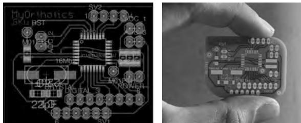
Figure 19. Schematic and proto board of the MyOrthotics Sku board
