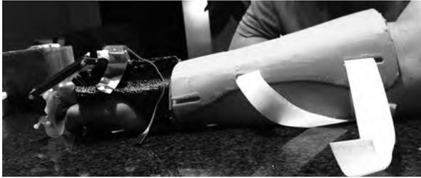
Figure 16. Testing the part and the interaction of the Myoware connection of the Myoware to the SatshaKit and assembling the Satshakit + Myoware + Motor + Orthotics Prototype. [https://youtu.be/\\_kyQ4P8TT0I](https://youtu.be/_kyQ4P8TT0I)
